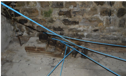
New blue rope pulley system
